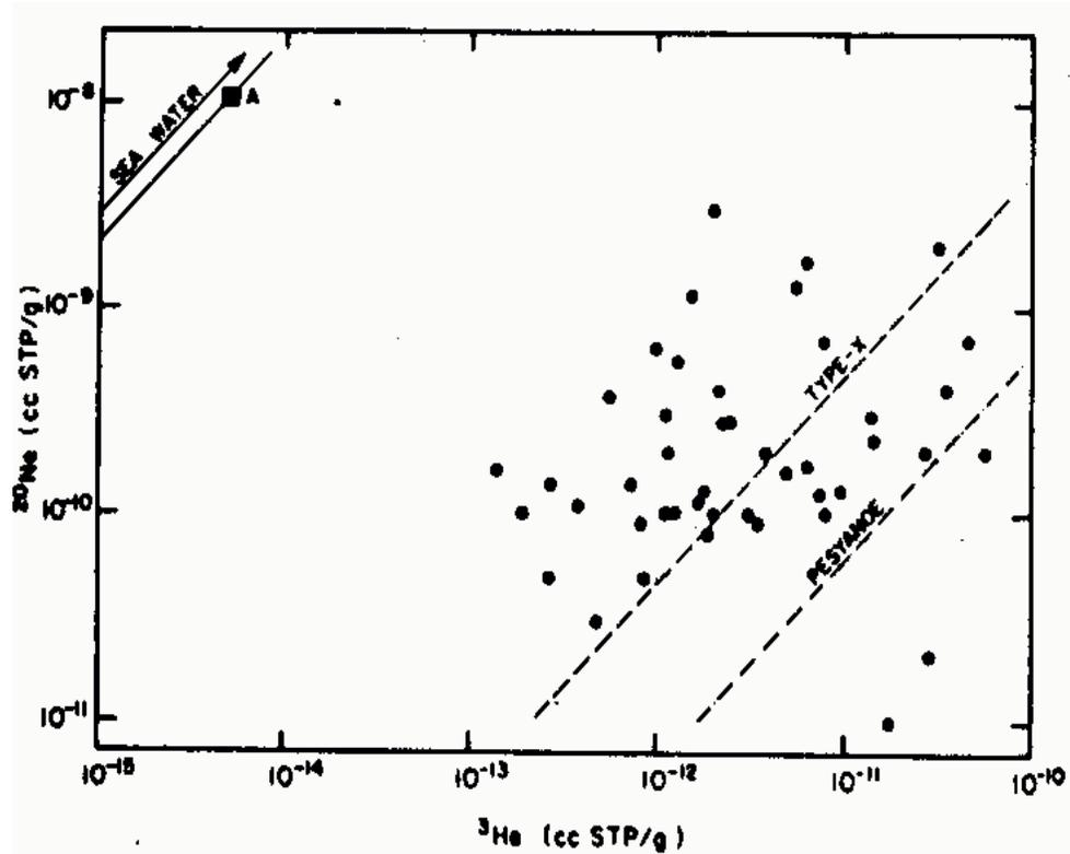
Fig. 4. Concentrations  $^{20}\text{Ne}$  and  $^3\text{He}$  in deep-seated samples ( $\bullet$ ). The bulk of these samples are enriched in  $^3\text{He}$  by several orders of magnitude, but depleted in  $^{20}\text{Ne}$ , relative to atmospheric gases. There is no apparent correlation of  $^3\text{He}$  and  $^{20}\text{Ne}$  concentrations. Point A and the lines are defined in the earlier figures.
