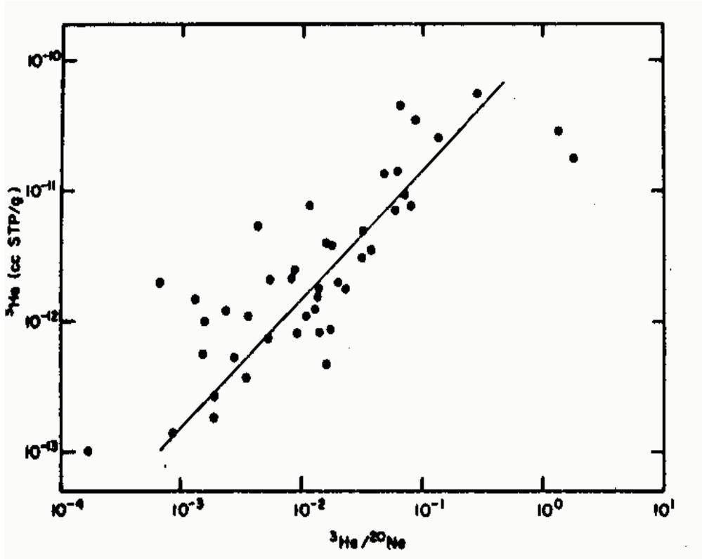
Fig. 6. Concentrations of  $^3\text{He}$  and values of the  $^3\text{He}/^{20}\text{Ne}$  ratio in deep-seated samples ( $\bullet$ ). The  $45^\circ$  correlation of the data indicates separate sources for the  $^3\text{He}$  and  $^{20}\text{Ne}$  contents.
